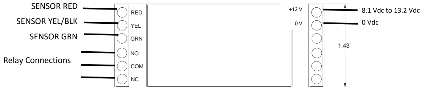
Figure 1. Wiring Connections - 14 AWG to 22 AWG
